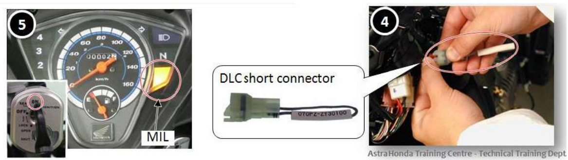
Gambar 3. 5 Pemasangan DLC short connector
